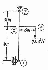
Use Castigliano's theorem (the least work theorem) to analyze the structure shown. Calculate the maximum bending moment and shear in the beams. The beams have EI = 9600 kN.m² and they are continuous from 1 to 3. The beams and strut 2-4 are inextensible. The tension bars 1-4 and 4-3 have EA= 25000 kN.
