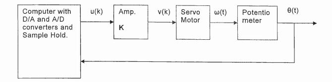
Where, u(k) is the output of the computer's D/A converter and sample hold. The voltage v(k) is the output of the amplifier (i.e. v(k) = Ku(k)). The angular velocity of the servo motor is  $\omega(t)$  and the output of the potentiometer is the angular position given by  $\theta(t)$ . You have a model of the servo motor given by the diagram,
