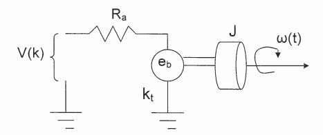
Where  $k_t$  is the motor torque constant in N-m/Amp,, J is the polar moment of inertia, R is the armature resistance. You are told that the motor must go to its commanded position within ½ sec and hold that position with a 0.5 degree accuracy. We know the following values,  $k_t$ = 1.0 N-m/Amp, J = 0.1 kg·m² and R = 10  $\Omega$ . Discuss your design consideration with regard to the following issues,
