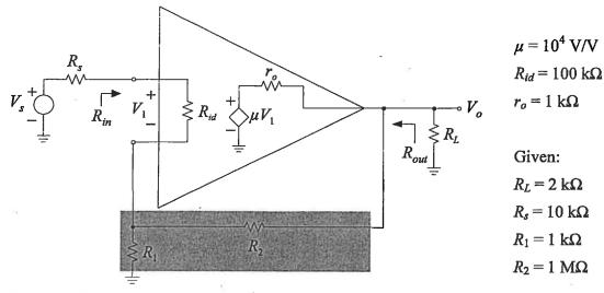
Using feedback theory, determine the following parameters:
