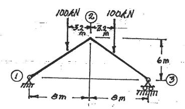
Use Castigliano's theorem (the least work theorem) to analyze the structure shown. Calculate the maximum and minimum bending moments on the beams (Minimum moments are frequently negative values). The beams have  $EI = 1.0 \times 10^5 \text{ kN.m}^2$ . and are inextensible. The tension bar has  $EA = 5.0 \times 10^3 \text{ kN}$ .
