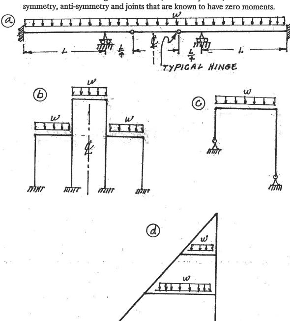
(12) 2. Schematically show the shear force and bending moment diagrams for the following structures. All members have the same EI and are inextensible.
