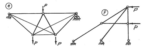
(18) 2. For each structure shown, compute the reactions and draw shear and bending moment diagrams. Indicate which are positive and which are negative segments of each bending moment diagram. For each shear and bending moment diagram, calculate and indicate the magnitudes of the maximum positive and negative ordinates.
