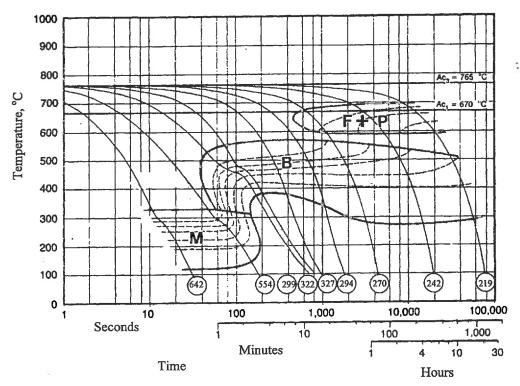
Considering the TTT diagram for a hypo-eutectoid steel, presented in the Figure above, calculate the cooling rates needed, in order to obtain 1) a F+P (ferrite and pearlite) microstructure with a hardness of 242HB, and 2) a fully martensitic (M) microstructure of hardness 554HB. (HB = Brinell Hardness scale)
