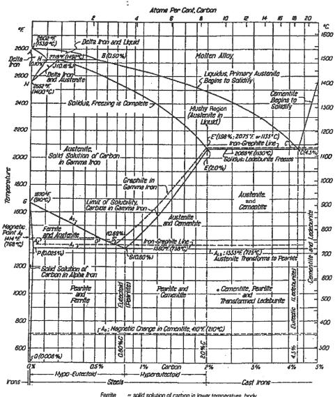
Ferrite = solid solution of carbon in lower temperature, body centered cubic form of iron.
