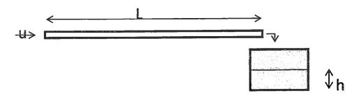
A pipe of length L=10 m is feeding liquid into a tank. The speed of the liquid in the pipe is u=1 m/s. The level of liquid in the tank is h. The cross section area of the tank is A=1 m<sup>2</sup>.
