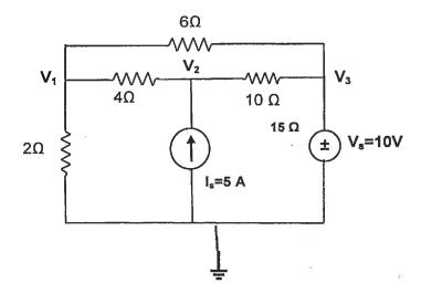
Q3: Write three mesh current equations in terms of  $I_1$ ,  $I_2$  and  $I_3$  in the following circuit and solve the current, I, flowing through the  $2\Omega$  resistor. [8+3+3+3]
