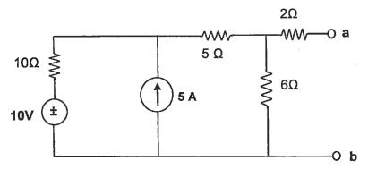
O2: In the following circuit, solve node voltage V<sub>1</sub>, V<sub>2</sub> and V<sub>3</sub> using nodal analysis. Use the bottom node as the reference node.
