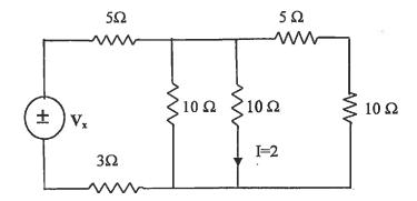
Q1(B): Find Thevenin equivalent circuit at terminals a-b of the circuit shown below . [6]
