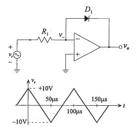
The op amp in this circuit is ideal except for a slew rate limit of  $0.5V/\mu s$ . It is powered by  $\pm 15V$  supplies. Given that
