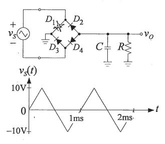
Due to an abnormal operating condition, Diode  $D_1$  in this full-wave rectifier circuit was suddenly destroyed, and stopped conducting in both forward and reverse directions (i.e. open circuit).
