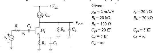
d) Find the mid-band voltage gain  $v_{OUT}/v_i$ .
