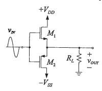
Given:  $K = 500 \text{ mA/V}^2$ ,  $V_{TH} = 1.0 \text{ V}$ ,  $R_L = 8 \Omega$  and  $|V_{DD}| = |V_{SS}| = 10 \text{ V}$ .
