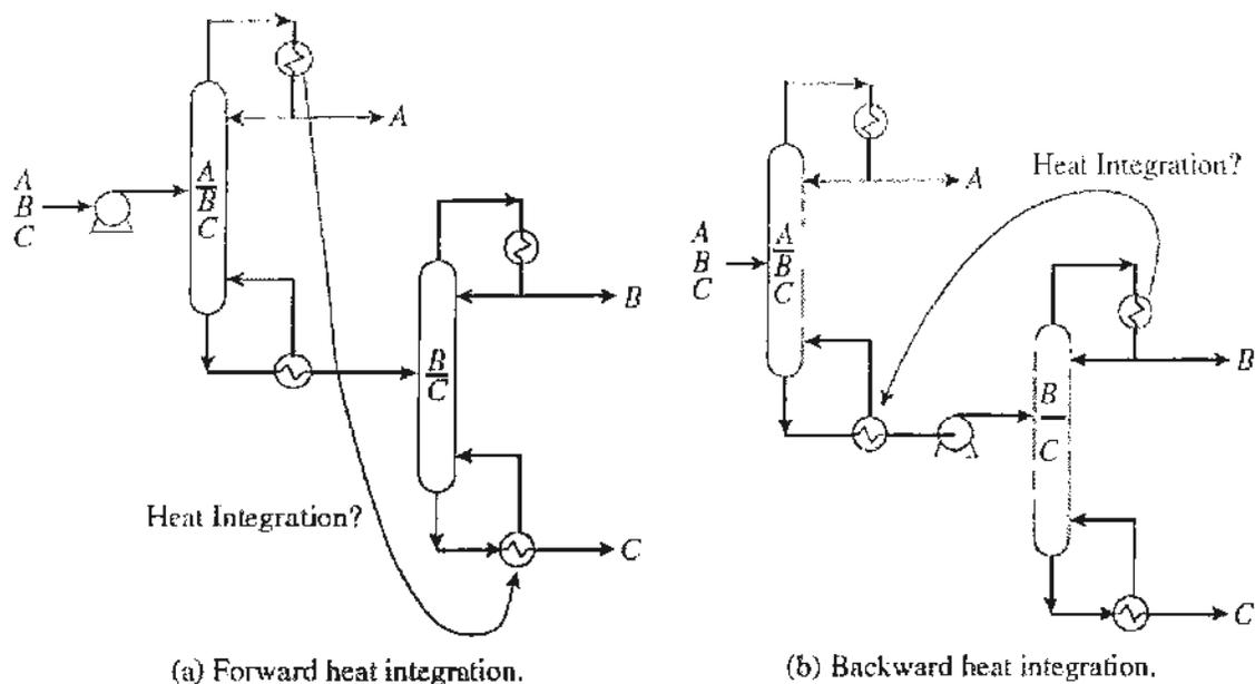
The operating pressures of the two columns need to be chosen to allow heat recovery. Data for Column #1 and Column #2 at various pressures are given below:
